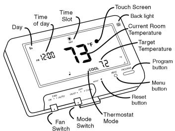
Statement of use: The 8085 can be used with most 24 volt gas, oil or electric heating and air conditioning systems, single-stage heat pumps or gas millivolt heating systems. It cannot be used with 120 volt heating systems or multistage heat pumps.
