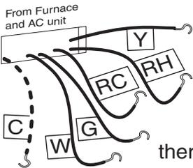
**STEP 1** - Remove the orange Jumper wire.
