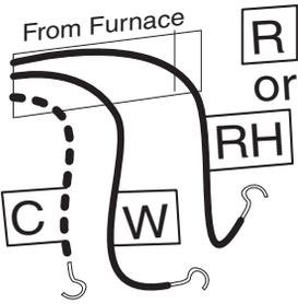
**STEP 1** - Connect the **R** (or RH) wire to the **RH** terminal on the thermostat.
