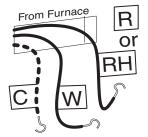
**STEP 1 -** Connect the **R** (or RH) wire to the **RH** terminal on the thermostat.
