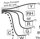
STEP 1 - Connect the Y wire to the Y terminal on the thermostat. This connects to the Cooler compressor.
