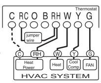
STEP 4 - Connect the G wire to the G terminal on the Thermostat. This connects to the Fan.
