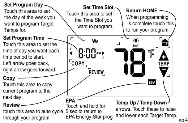
NOTE: The Mode Switch must be in HEAT or COOL mode to configure.
