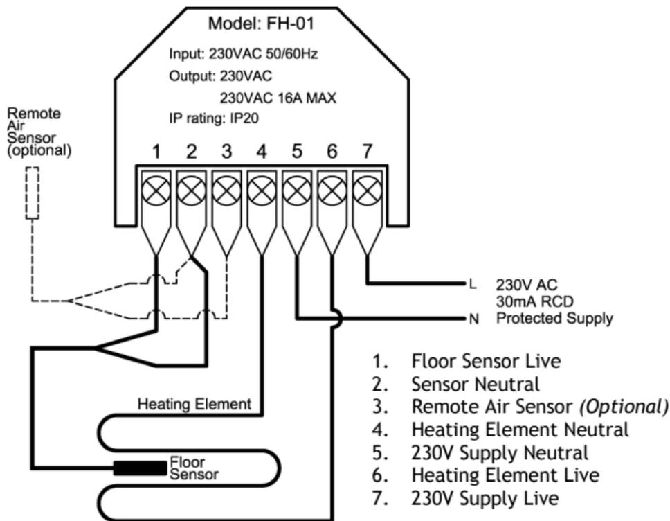
*nb: generally underfloor heating elements are not polarity conscious, in such cases the heating element can be connected to the live and neutral either way round, unless insulation colouring dictates otherwise.*
