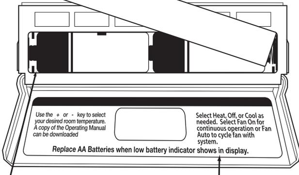
Insert 2 AA Alkaline batteries (included). High quality alkaline batteries are recommended.
