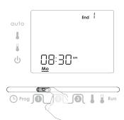
2- Turn the dial to set the time. Move the Program slider to the next position to confirm/finish this setting.
