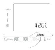
2- Press and hold Enter for 5 seconds to access the setting mode.
