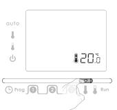
2- Turn the dial to set the temperature between 5°C and 30°C, in increments of 0.5°C.
