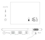
4- Turn the dial to set the temperature between 5°C and 30°C, in increments of 0.5°C.
