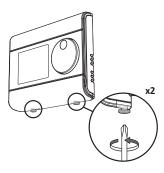
**2-** Remove the wall plate from the thermostat.
