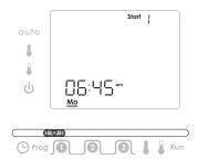
4- Turn the dial to set the time. Move the Program slider to the next position to confirm/finish this setting.
