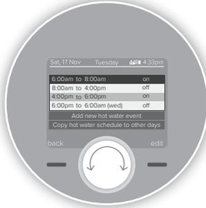
Push the dial to edit a hot water time or temperature when it is highlighted in light blue. You can also add an additional heating period by scrolling and pushing on the “Add new hot water event” bar. You can have up to 6 hot water events per day in your schedule.
