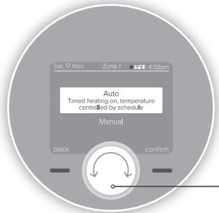
Use the dial to scroll between the different modes (Auto, Manual and Off) and then push the dial or press the right hand button to confirm your selection
