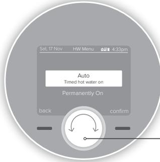
Use the dial to scroll between the different modes (Auto, On and Off) and then push the dial or press the right hand button to confirm your selection
