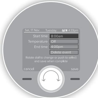
Alter the start and end times of the hot water period and the temperature by scrolling the dial to then pushing the dial to edit. Then use the dial to alter the time or temperature and push to confirm. Push the dial or the right hand button to save your changes.
