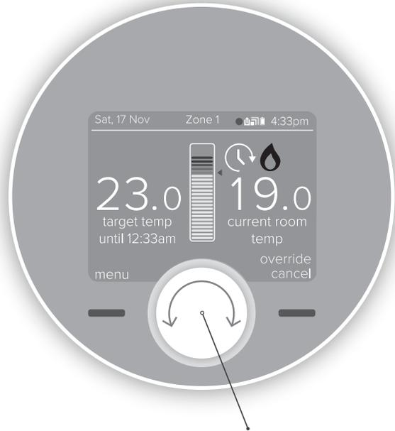
Turn the dial to adjust the target temperature temporarily (this could be up or down)
