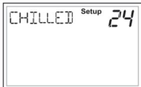
These steps configure the type of water valve(s) connected to the thermostat. A normally closed valve allows no water flow when no power is applied to it. A normally open valve allows water flow when no power is applied to it. Some 4 pipe fancoils use a normally closed chilled water valve with a normally open hot water valve. If you have a two pipe fancoil, the setting in Setup Step 24 for CHILLED WATER VALVE will apply to the single valve in use.
