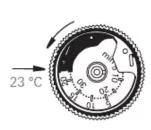
4. To set the blue setting ring to the lower temperature limit (8 °C here): Insert a pointy object (e.g. pen) into the hole of the blue ring. Rotate the blue ring clockwise to 8 °C.
