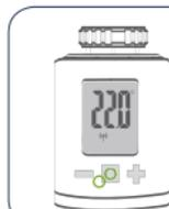
After successful installation **press the green blinking button** to start the adaption. Once the adaptation is completed, the display shows the setpoint temperature.
