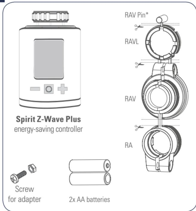
\* When using the RAV adapter, you need the RAV Pin for the extension of the valve stem.
