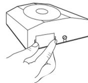
Remove the battery compartment by pinching the tabs and withdrawing downwards. Replace the spent batteries with 2 x AA 1.5V alkaline batteries ensuring correct orientation. Replace the battery compartment pressing fully home.
