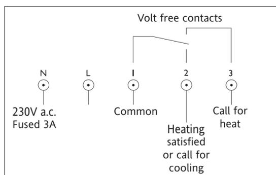
This product is double insulated and does not require an earth connection. The SCR should be wired to the combi boiler or central heating wiring using the correct type of cable or flex. The SCR should be wired in to replace hard wired room or programmable thermostats shown on the system or boiler wiring diagrams. Always check other manufacturers instructions for compatibility.
