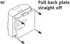
To wire the external sensor, snap out the cable entry strip on the bottom right edge of the thermostat cover.
