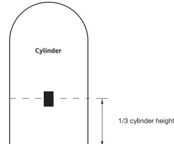
The plastic covered spring fixing cable should be cut to an unstretched length of approximately 60-75mm (2 1/2"-3") less than the circumference of the cylinder and the hook and eyelet should be screwed into the ends. Stretch the cable round the cylinder, over the insulation, and position it in the groove across the front of the sensor housing. Engage the hook and eyelet.
