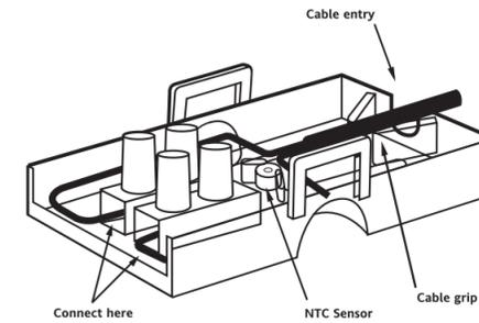
Clip the spacer provided onto the sensor housing.
