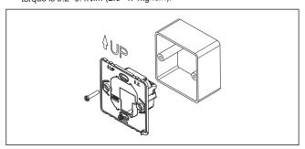
4) Re-mount the front cover via snap-fit connection.
