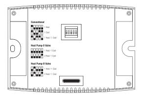
Install the control module near the heating/cooling system, away from any heat source.
