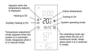
The controller normally displays the measured indoor temperature. To view the setpoint, press one of the ▲▼ buttons. The setpoint and the ▶ symbol will be displayed for the next 5 seconds.
