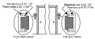
Secure the wallplate to the electrical box using 6-32, 1/2" screws. See above drawing
